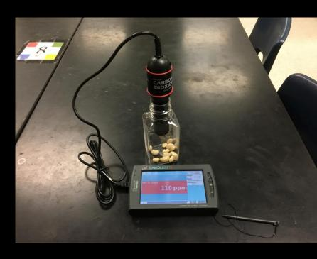
Press the green arrow on the bottom left side of the LabQuest, this will start an new experimental data collection.
