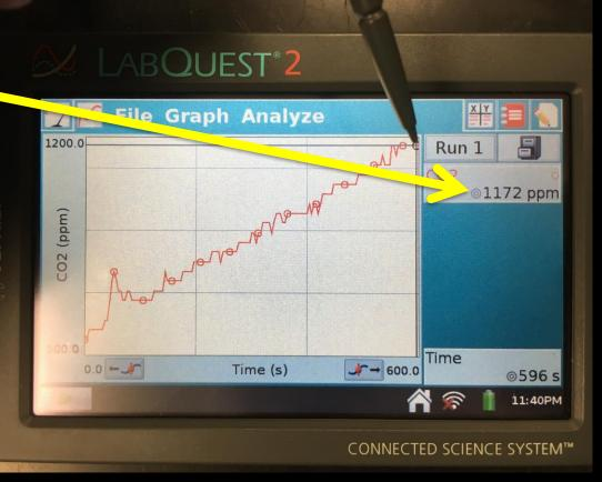
Subtract the starting level from the ending level to get the CO<sub>2</sub> Produced
