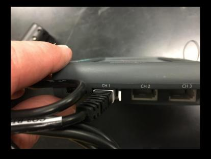
The LabQuest will automatically detect that you have inserted a CO<sub>2</sub> probe. The screen should change and you will start to see CO<sub>2</sub> readings in Parts Per Million (ppm)
