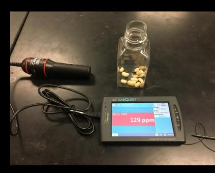
Place the CO<sub>2</sub> Probe into the Reaction Bottle
