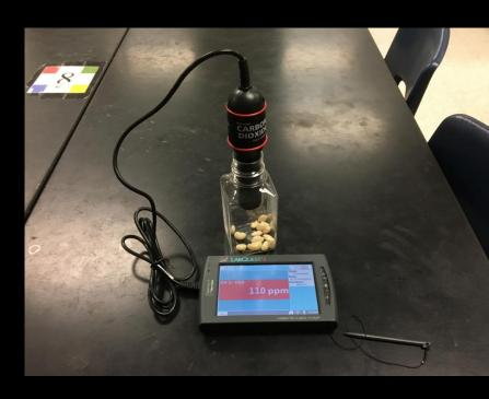
Press the green arrow on the bottom left side of the LabQuest. This will start the data collection for your first experiment.
